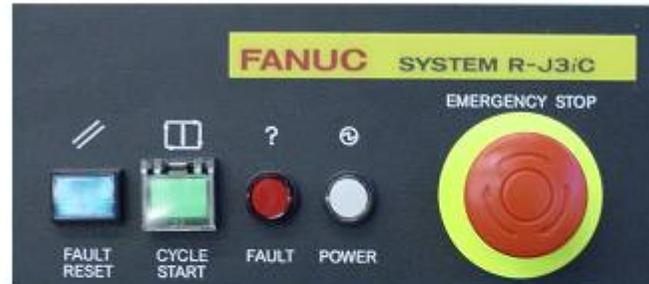
Standard Operator Panel (SOP) R-J3iC
